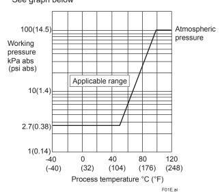
Figure 1. Working Pressure and Process Temperature
