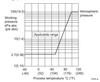
Figure 1. Working Pressure and Process Temperature
