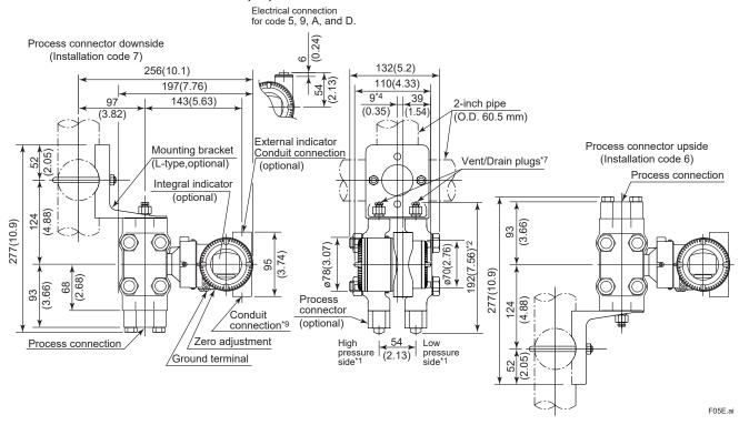
Horizontal Impulse Piping Type (Installation code 9)
