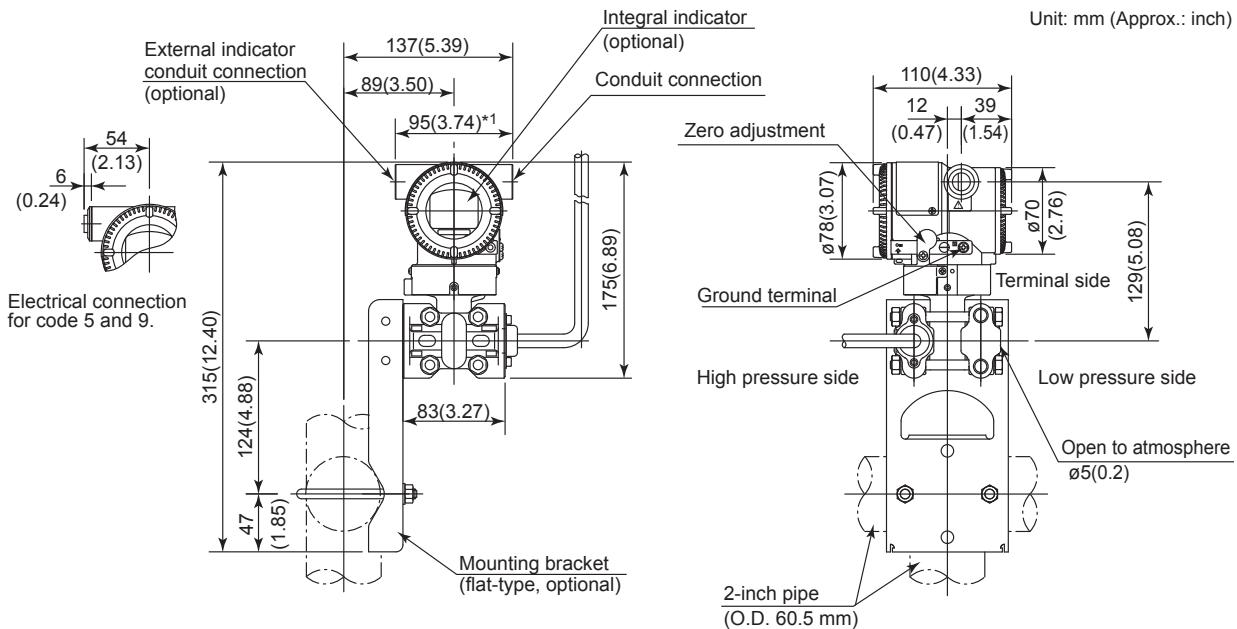
\*1: When electrical connection code 7 or C is selected, a blind plug is protruded upto 8 mm (0.31 inch) from the conduit connection.
