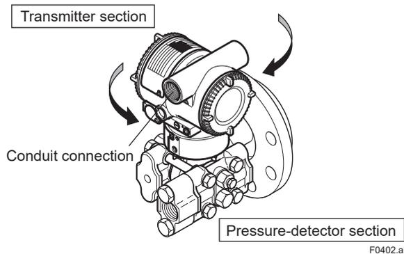
Figure 4.2 Rotating Transmitter Section
