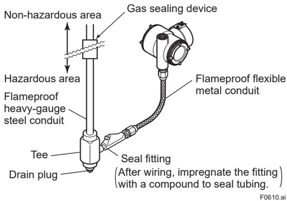
**Figure 6.15 Typical Wiring Using Flameproof Metal Conduit**
