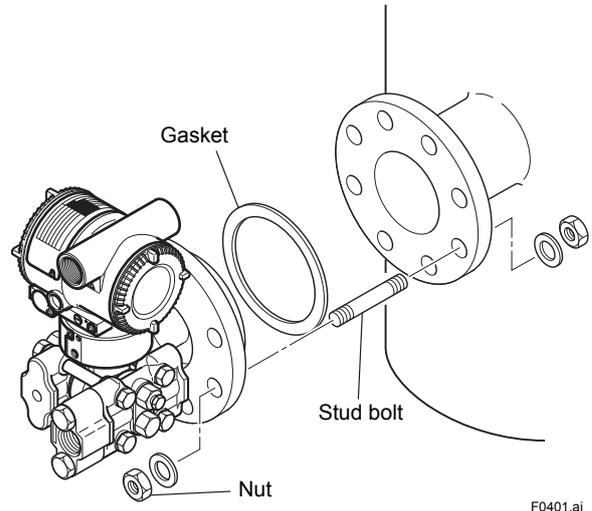
Figure 4.1 Transmitter Mounting
