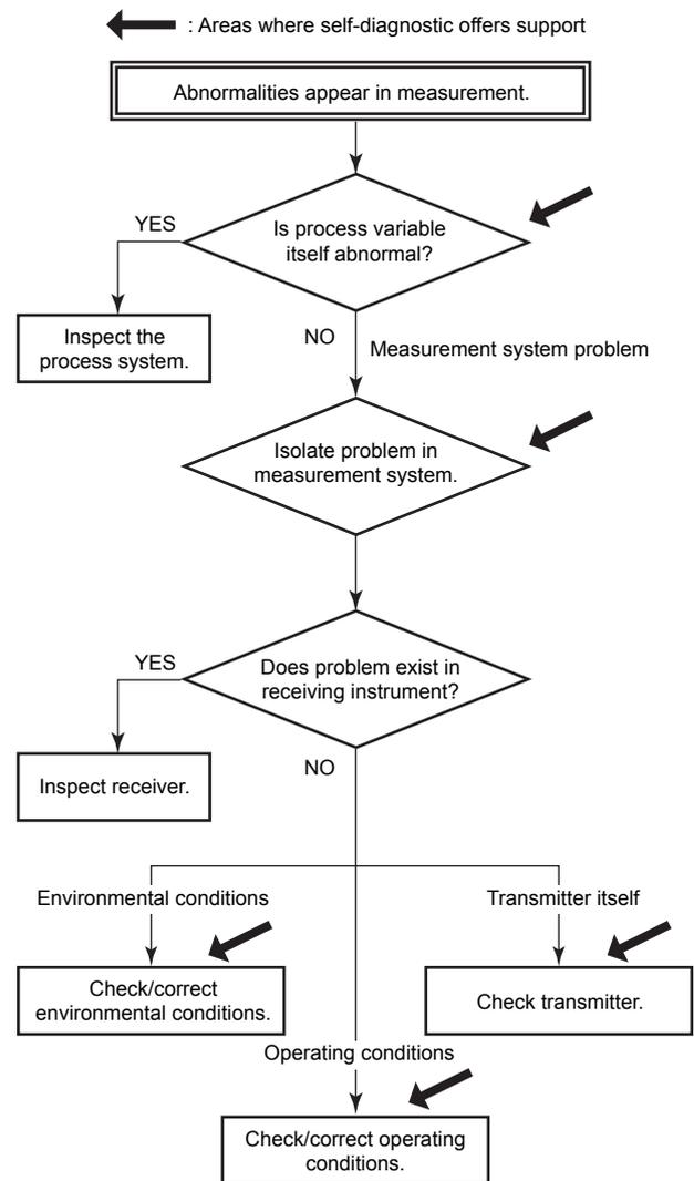
Figure 8.5 Basic Flow and Self-Diagnostics
