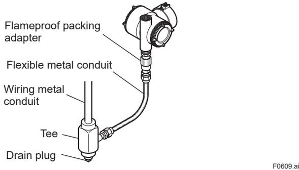
**Figure 6.14 Typical Cable Wiring Using Flameproof Packing Adapter**
