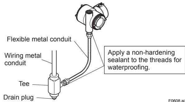
**Figure 6.13 Typical Wiring Using Flexible Metal Conduit**
