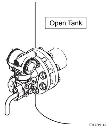
Figure 7.1 Liquid Level Measurement
